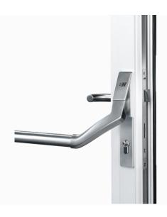
With its series **BDE-D2500** (touch bar), the **BLUE WEST** Premium project door furniture and corresponding complementary accessories, **BLUE WEST** is able to offer a high-performance panic hardware system ideal for both internal and external timber door applications. The integrated mortise panic/emergency escape lock enables the door to be engaged by both latch and bolt.
