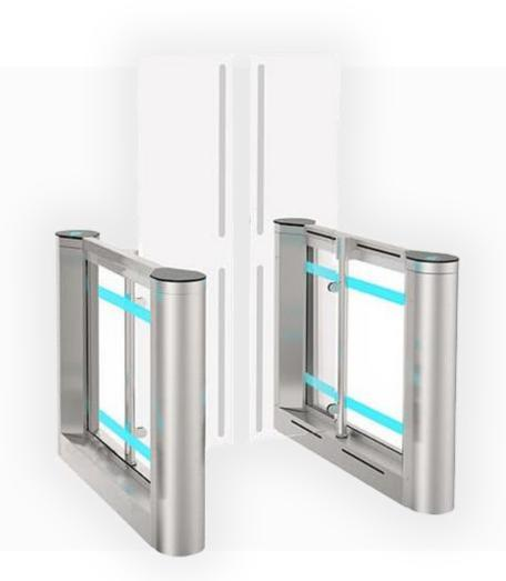
Tall version of speed gates model intended for applications where a higher degree of security is required. High swing glass leaves available up to 1800 mm from the floor. It helps to avoid transfer of anything above the turnstile, as well as overjumping it. Special design allows to arrange even 900 mm passage which can be used for people with special.
