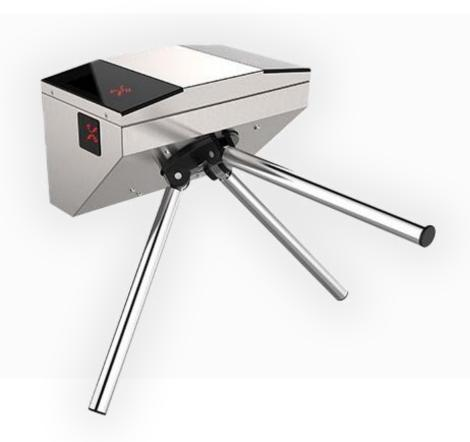
**BW-SKULL-M** is a gate barrier with a special wall mounting design. BW-Skull-M turnstile has a double LED indication - on the side and on top. A variety of housing finishing types enables this tripod turnstile to be fitted to a range of installation sites, both indoors and outdoors. It includes an anti-panic function (to prevent injury in the case of people panicking by allowing fast and easy egress to the people in the building).
